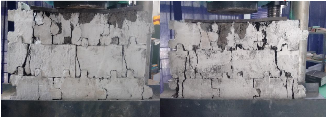
Figure:6 failure of conventional mix
